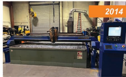
10' x 25' Machitech Gold Cut Plasma Table, with HPR400HD
